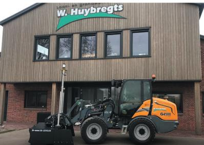
Huijbregts is always looking for new possibilities. A great example was their idea to revamp an existing leveling attachment. Their request: turn it into a state-of-the-art leveler for soccer pitches and other large surface areas with vertical and horizontal control based on GNSS.
